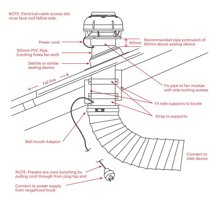
Recommended minimum duct length 3m. Extend flexible ducting. Cut to length.
