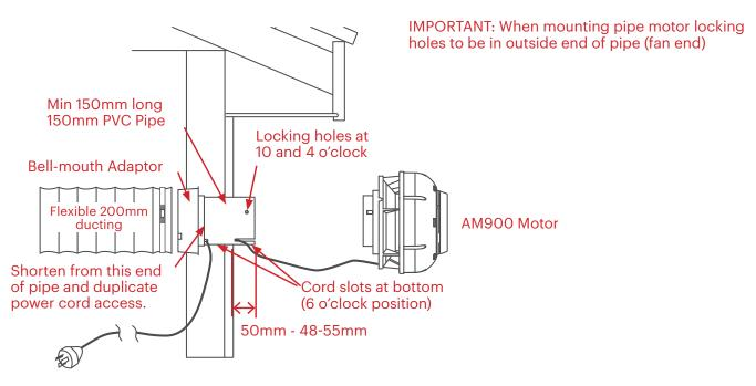
NOTE: Ensure that power cord is fed through exit slot and is not allowed to double back restricting motor inlet.
